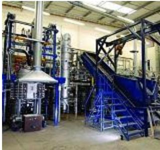
In collaboration with Advanced Plasma Power (AAP) and Progressive Energy, the company aims to demonstrate the use of waste to produce bio-substitute natural gas (Bio-SNG) using a process called Gasplasma.
