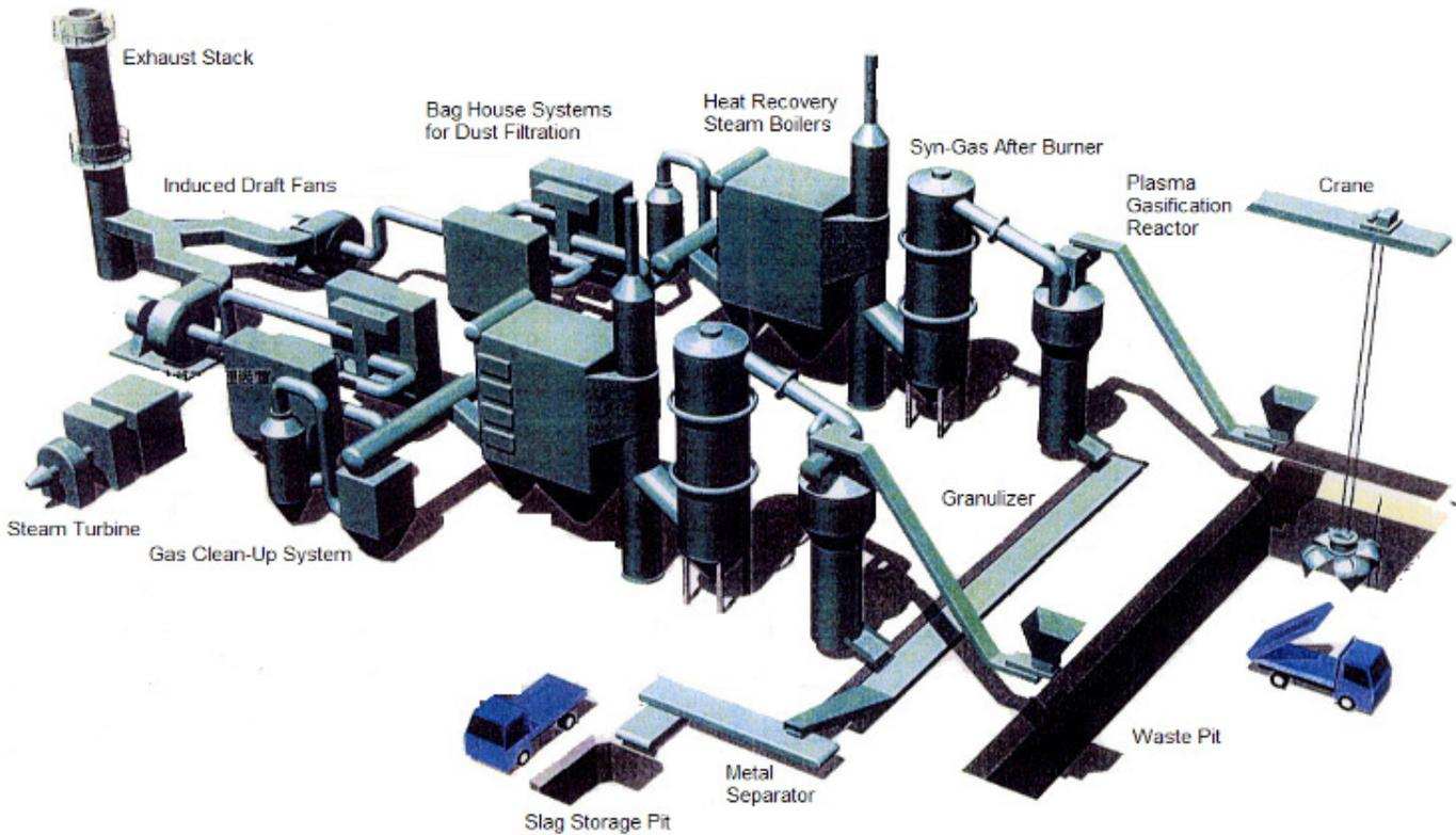
**FIGURE 2 - PROCESS FLOW FIGURE FOR ECOVALLEY MSW AND ASR GASIFICATION FACILITY**
