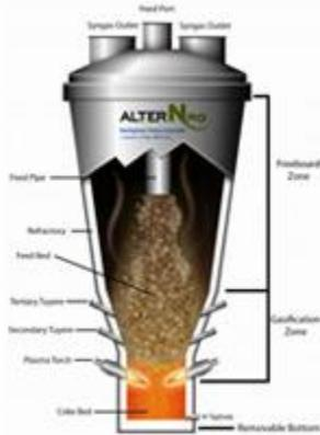
The waste then is passed through an airlock which prevents gases from escaping into the atmosphere. The plasma gasifier is an insulated air-tight container with plasma torches at the base to provide the heat required to gasify the waste feed. The plasma torches consume a very small portion of the total energy available from the feedstock (2-5% of total energy input) in providing part of the heat required to drive the endothermic gasification process.
