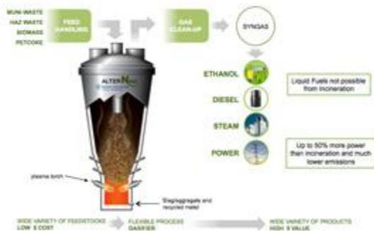
The Plasma Gasifier produces a gaseous product and an inert solid by-product; the individual amounts of which will depend on the type of waste being feed into the gasifier.
