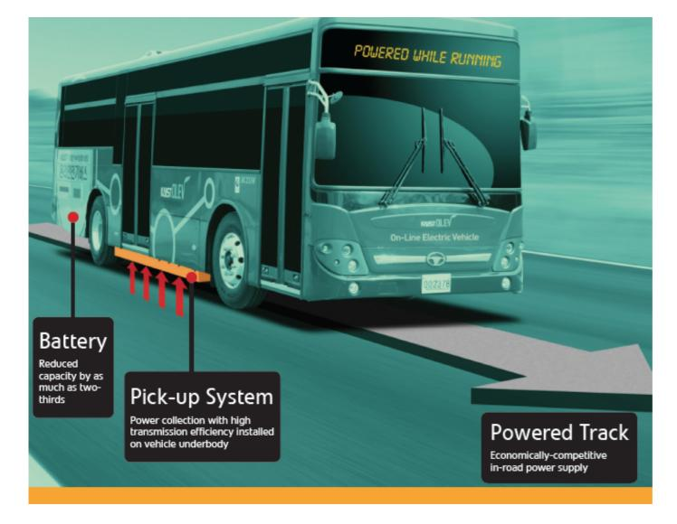
Last August, OLEV Korea set up its system for two buses in Gumi, South Korea, each running a continuous 24 km inner-city route. As an example of a typical application of the OLEV charging system, charging apparatuses are installed beneath the street in strips of concrete-encased wires 5 m at a time. The wires create the inductive charge, and when needed are placed in series, as in the case of "take-off segments" – 20 m strips that provide an extra lift for accelerating up hills.
