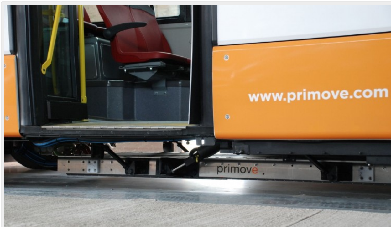
12m Solaris battery-electric bus with the PRIMOVE inductive charging system from Bombardier
