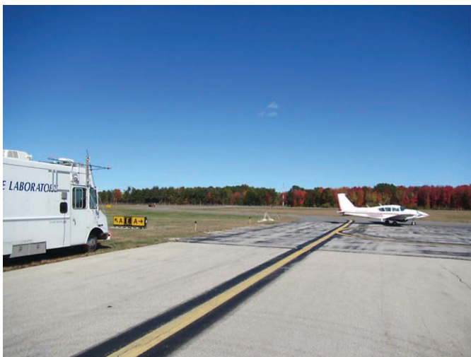
Figure 2-4. Ideal geometry for engine testing. The aircraft test is performed next to an unused taxiway. The exhaust and propeller wash are directed into an open field with no buildings or aircraft. The probe is placed just off the taxiway. The measurement equipment (the white truck) is out of the way.
