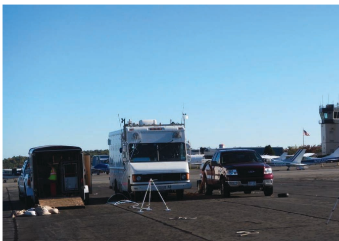
Figure 2-3. Measurement setup. The tow-behind trailer to the left houses the particulate matter instrument suite. The white truck in the middle is the Aerodyne Mobile Laboratory, housing the gas-phase instrumentation and data acquisition computers. The red truck to the right is towing a construction generator that powers all the instrumentation.
